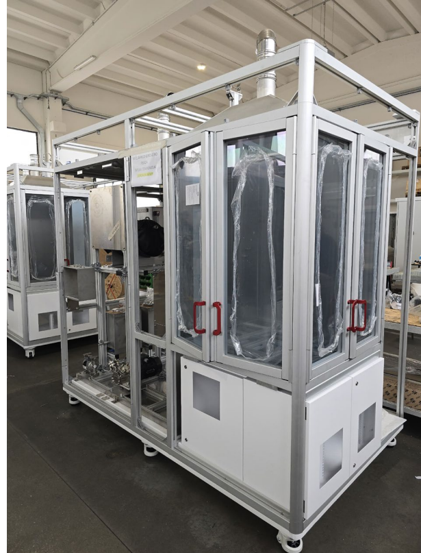
Frame of first two test benches (AEM, AEL) assembled
