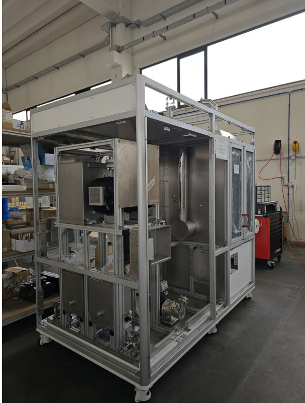
Frame of first two test benches (AEM, AEL) assembled
